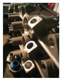
The 12 mm hole is the one on the bottom and the stock rail is the one on the top. The M12 fitting (blue one) is show next to the 1/8" npt fitting in the bottom left corner of the picture.
