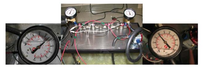
The setup varied only slightly when flow measurements were taken. Two graduated cylinders were attached to the upstream (pump side) injector and the downstream (FPR side) injector. The
