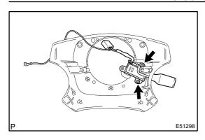
(d) 4 spoke steering wheel assy: Remove the 2 screws and cruise control main switch assy.
