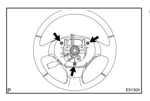
(f) 3 spoke steering wheel assy: Reverse the steering wheel, remove the 3 screws and cruise control main switch assy.
