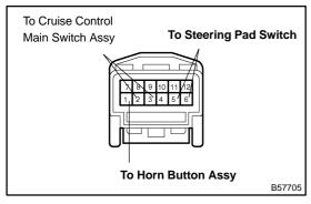
(g) Disengage the wiring pins other than the cruise control main switch assy from the connector, and pull them out.
