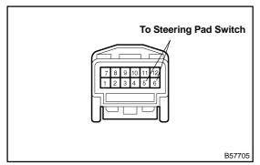
(c) Disengage the wiring 2 pins from the connector, and pull them out.
