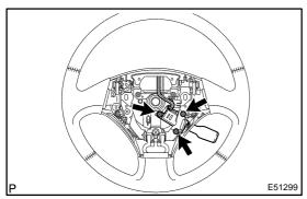
(e) 3 spoke steering wheel assy: Remove the 3 screws.
