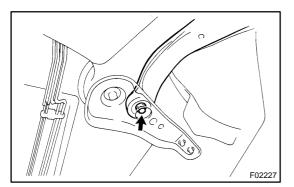
Install the front suspension arm sub-assy lower No. 1 LH with the bolt and nut to the rear side.
