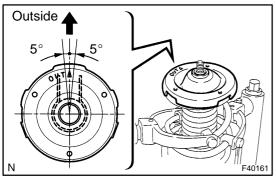
(f) Install the front coil spring seat upper LH to the shock absorber assy front LH with the mark facing to the outside of the vehicle.
