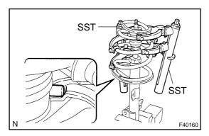
(c) Using SST, compress the front coil spring LH. SST 09727–30021
