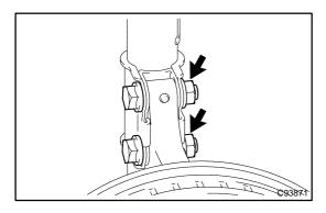
(c) Install the 2 bolts and 2 nuts to the lower side of front shock absorber with coil spring.
