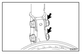
(d) Remove the 2 nuts and 2 bolts on the lower side of front shock absorber with coil spring.
