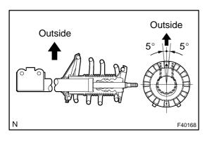
(e) Install the front coil spring insulator upper LH as shown in the illustration.
