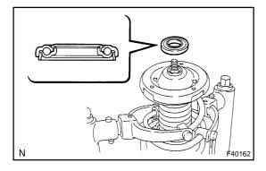
(g) Install a new front suspension support bearing LH.
