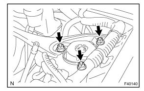
(b) Install the 3 nuts to the upper side of front shock absorber with coil spring.
