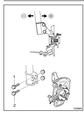
(e) Adjust the camber by pushing or pulling the lower side of the shock absorber in the direction in which the camber adjustment is required.
