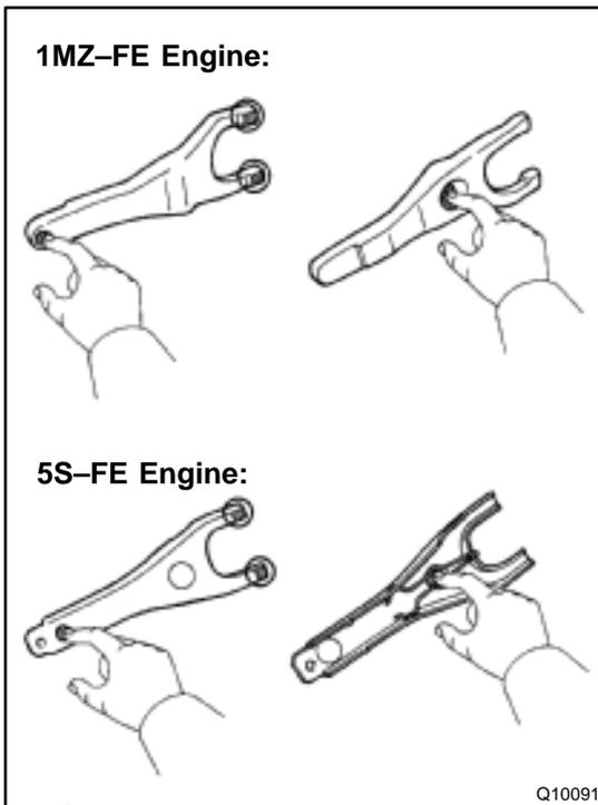
**3. APPLY MOLYBDENUM DISULPHIDE LITHIUM BASE GREASE (NLGI NO.2)**
